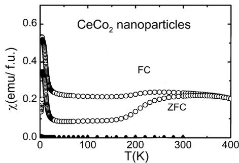
Fig. 2. ZFC and FC magnetic susceptibility of CeCo<sub>2</sub> nanoparticles under  $H = 200\text{ G}$  (open circles) and the magnetic susceptibility of CeCo<sub>2</sub> bulk under  $H = 1000\text{ G}$  (solid circles).
