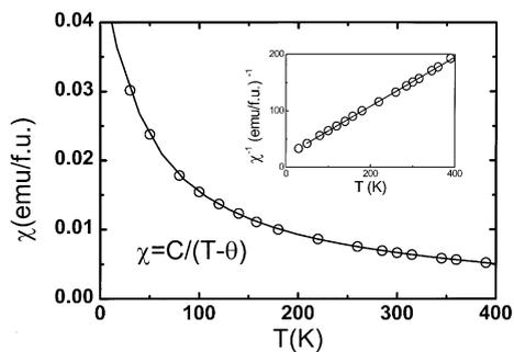
Fig. 4. The extracted  $\chi$ 's fitted to a Curie–Weiss law represents a paramagnetic phase in  $\text{CeCo}_2$  nanoparticles.
