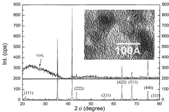
Fig. 1. The X-ray diffraction patterns of CeCo<sub>2</sub> nanoparticles (the top) and CeCo<sub>2</sub> bulk (the bottom). The bump at  $2\theta \sim 20\text{--}35^\circ$  is the background of grease for sample attachment. A blurred anomaly around  $2\theta = 28.6^\circ$  on top of the background corresponds to the main (111) peak of CeO<sub>2</sub>; inset: the HRTEM image of CeCo<sub>2</sub> nanoparticles.
