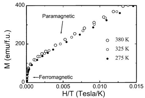
Fig. 3. The magnetization of CeCo<sub>2</sub> nanoparticles versus  $H/T$  for several temperatures.
